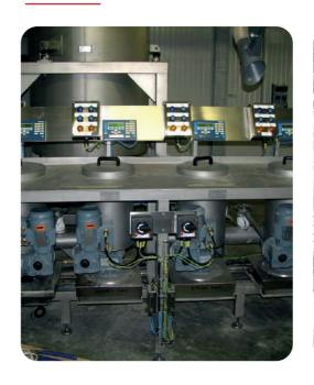
TRANSITUBE has developed several sets of equipment allowing to carry out a dosage of each product (powders, granules or aggregates) via the flexible screw and depending on the different required ratios.
