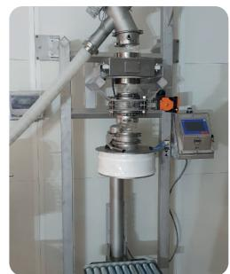
Bagging weighing system for packaging powdered and granulated bulk products in drums or open bags
