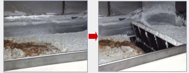
Example of automation with a driven flap for remelting
